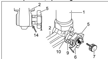
**Unlocked position, ball bar not mounted**
