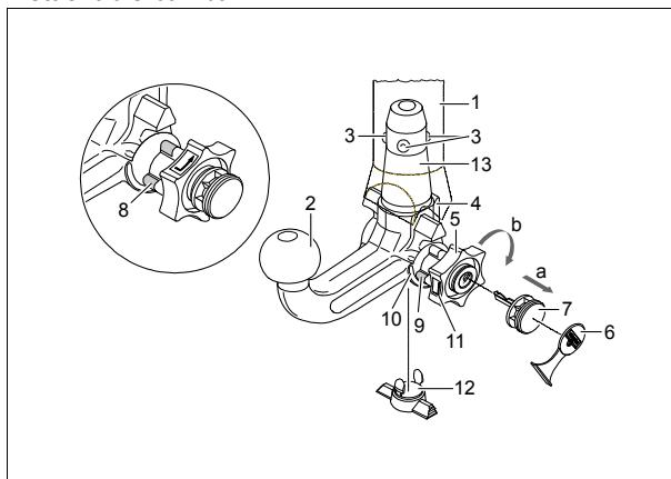
**Locked position, operating condition**
