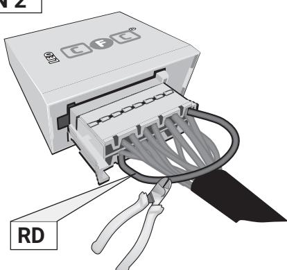
Pin 11 and Pin 2 disconnected
