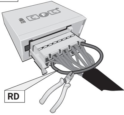
Pin 11 and Pin 2 disconnected
